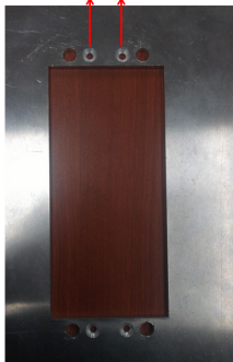
M4 countersink screw hole
